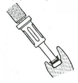
Locator Core Tool Removal Tip – Tip End Fig 5
