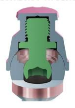
This revolutionary, patent-pending retention system works similar to a ball and socket, allowing the Denture Attachment Housing to securely snap into place and then pivot to the desired position. Once in place, it's fixed for the patient, and can easily be removed by the clinician at hygiene and maintenance visits.
