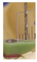
2. The 1.7mm Bar Drill #9102 and a 2.0mm Bar Tap #9104 are used for creating the threaded site in a titanium bar or cast alloy bar.
