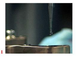
3. Use the 1.7mm Bar Drill (#9102) in a precision drilling device to create the exact size diameter hole to a <u>depth of 2.8mm</u> that is needed for tapping the site (**FIG 2**).
