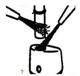
Make a hole to allow investment to fill the space and pass through (FIG 6). Invest, cast, and devest. Thread the fixation screw into the tube to act as a handle. Clean the outside of the tube of any body oils. Sandblast the outside of the tube and the space in the casting with clean, small size, aluminum oxide (FIG 7). Clean the outside of the tube and the inside of the space in the casting.
