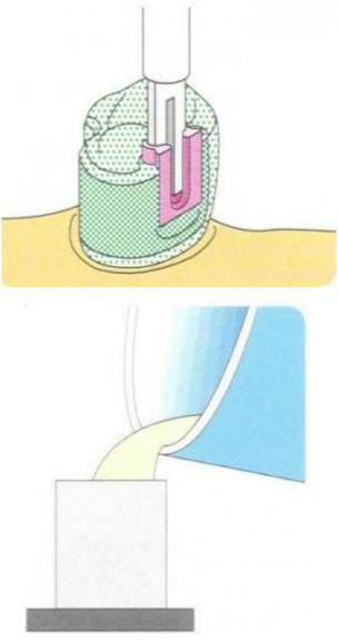
Due to the swelling affect of plastic, wax ups with integral plastic slide attachments should be invested in a phosphate-bonded precision investment compound.
