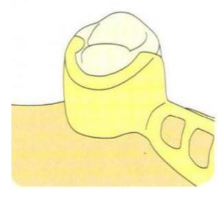
Free end situations require a lingual milled brace support in order to protect the slide attachment. Wax up the abutment crown as desired and integrate the appropriate female part in the wax up using the Paralleling Mandrel.
