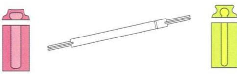
Use the Paralleling Mandrel for both of the Female Parts of the Dupla Attachment–The Rod Female Part (green) and the T-shaped female part (pink). When using the Pink T-shaped component, make sure that the Paralleling Mandrel activating slot is visible in the opening of the T-shaped female part.
