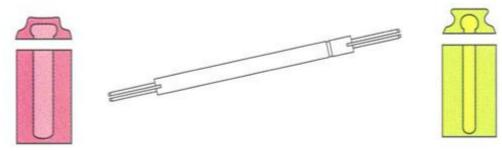
Use the Paralleling Mandrel for both of the Female Parts of the Dupla Attachment–The Rod Female Part (green) and the T-shaped female part (pink). When using the Pink T-shaped component, make sure that the Paralleling Mandrel activating slot is visible in the opening of the T-shaped female part.
