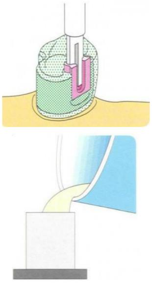
Due to the swelling affect of plastic, wax ups with integral plastic slide attachments should be invested in a phosphate-bonded precision investment compound.
