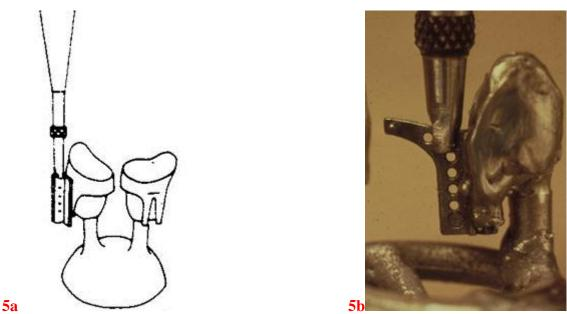
Invest and cast the crowns using the alloy of choice. Do NOT use a carbon containing investment. Burn out at 1700 degrees F with a one hour heat soak. When using a high palladium alloy, be careful not to overheat the alloy. Use an oxygen setting of 10psi when torch melting.
