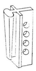
Two types of FR attachment males are available. Use the <u>Self Cure FR attachment</u> male (**FIG 7**) with the tail extension when no hinges are being used and/or the male is to be attached to the cast partial frame with self cure resin on the master model. The <u>Direct Cast FR attachment</u> male (**FIG 8**) without the tail is used in combination with the <u>DSE Hinge</u> and/or if a fixed connection or direct casting between the partial restoration and the saddle retention is preferred.
