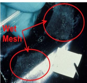
Every piece of Perma Mesh has been impregnated with PMMA via a silane coupler. Unique to Perma Mesh and eFiber is that these materials form a chemical, as well as mechanical bond, with resins.
