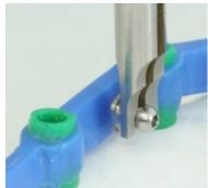
Do not sandblast to devest or use rubber wheels to polish the attachment. Glass beads, shells, or a PREAT fiberglass pencil work when devesting to maintain the accuracy of the male attachment. Lightly polish to a smooth finish.
