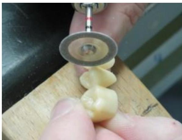
A special thin Disc is available for cutting of sprues and interproximal adjusting.
